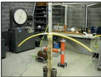
Setup of a dielectric test of the LPG-Flex pipe by a third party lab to meet the new EN 16125 Standard.
