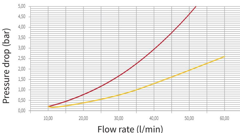
Plastics are about 100 times smoother than steel. The smaller LPG-Flex pipes will give identical flow results than the typically larger steel pipes.
